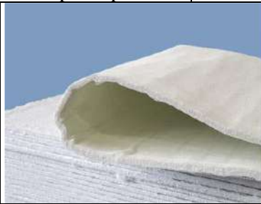
Fig. 4: Spaceloft fibers-reinforced blankets and Aeroplan Basic Aerogel (4) .
