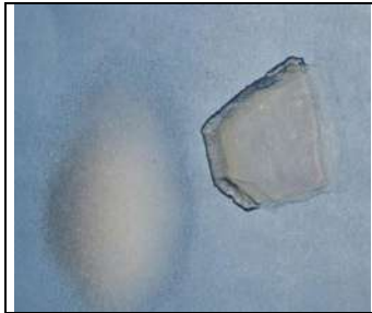
Fig. 3: Silica aerogels: monolithic pane (right) and granular (left) (5) .
