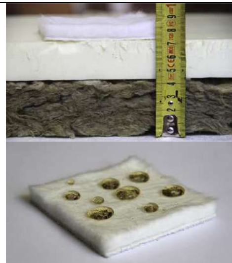
Fig. 9: Rock wool, polyurethane, and fiber-reinforced polymer thickness comparison (2)
