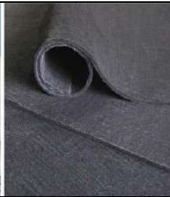
Fig. 4: Spaceloft fibers-reinforced blankets and Aeroplan Basic Aerogel (4) .
