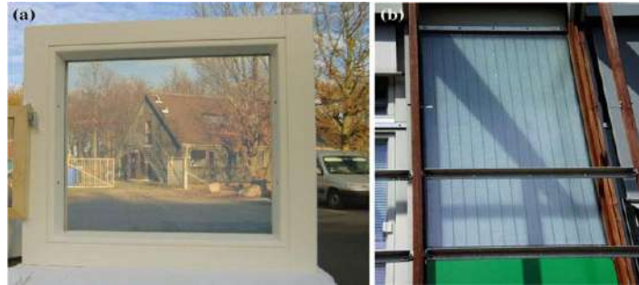
Fig. 11: a monolithic aerogel prototype; b a prototype of a PMMA system using granular aerogel.
