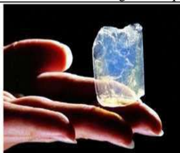
Fig. 6: Aerogel, the world's lightest solid (5)
