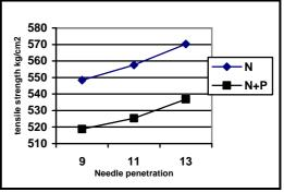
Fig. (2) Effect of fabric type and needle penetration depth mm on the tensile strength at break in the width direction at weight  $3400 \text{ gm/m}^2$
