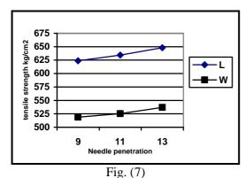
Effect of fabric type and needle penetration depth mm on the tensile strength at break in the two directions of the fabric type 75% Nomex + 25% polyester at weight 3400 gm/m<sup>2</sup>
