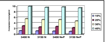
Fig. (20) Effect of fabric type and the weight  $gm/m^2$  on the compression force  $kg/cm^2$  (lost of thickness ratio %) at puncture depth 11 mm
