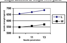
Fig. (5) Effect of fabric type and needle penetration depth mm on the tensile strength at break in the two directions of the fabric type 100% Nomex at weight  $3400 \text{ gm/m}^2$
