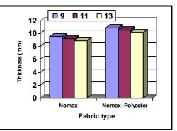
Fig. (26) Effect of fabric type and needle penetration depth mm on the thickness (mm) at weight  $3150 \text{ gm/m}^2$
