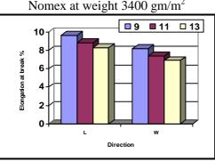
Fig. (15) Effect of fabric type and needle penetration depth mm on the elongation at break % in the two directions of the fabric type 75% Nomex
