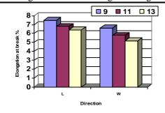
Fig. (13) Effect of fabric type and needle penetration depth mm on the elongation at break % in the two directions of the fabric type 100%
