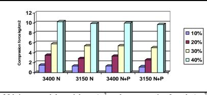
Fig. (21) Effect of fabric type and the weight  $gm/m^2$  on the compression force kg/cm<sup>2</sup>(lost of thickness ratio %) at puncture depth 13 mm
