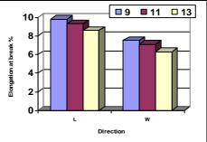
Fig. (14) Effect of fabric type and needle penetration depth mm on the elongation at break % in the width direction of the fabric type 100% Nomex at weight 3150 gm/m<sup>2</sup>
