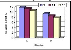
Fig. (16) Effect of fabric type and needle penetration depth mm on the elongation at break % in the two directions of the fabric type 75% Nomex
