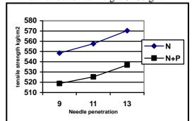
Fig. (4) Effect of fabric type and needle penetration depth mm on the tensile strength at break in the
