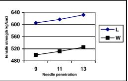
Fig. (6) Effect of fabric type and needle penetration depth mm on the tensile strength at break in the two directions of the fabric type 100% Nomex at weight  $3150 \text{ gm/m}^2$
