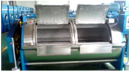
Figure (3) Side Loading Cellulase Washing Machine
