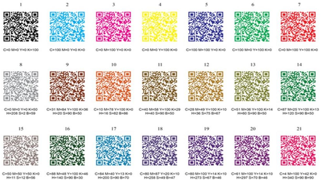
Figure 2: 21 patches of colored QR codes on digital file in pre-press stage
