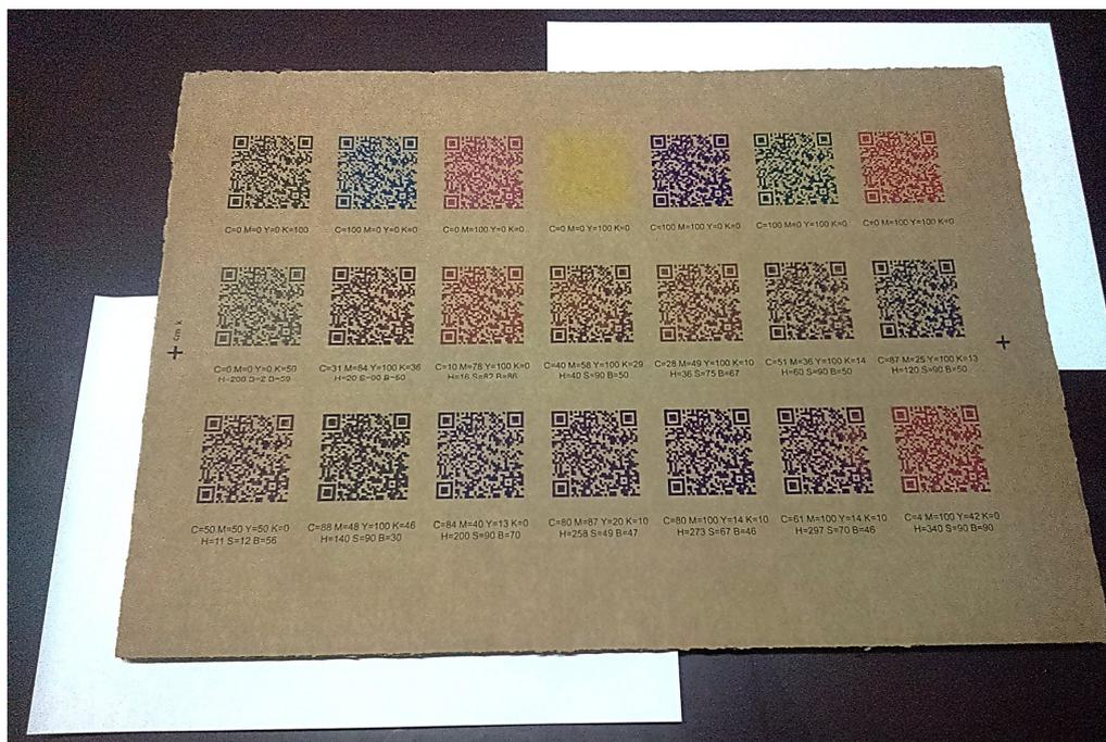
Figure 3: 21 printed patches of colored QR codes after printing on brownish corrugated board
