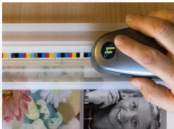
Figure (8): Using the long pressSIGN ruler to measure a full press sheet
