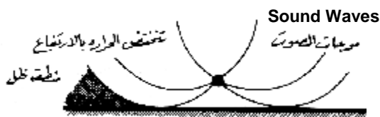
(Fig.19) illustrates spreading of sound waves during the day.
