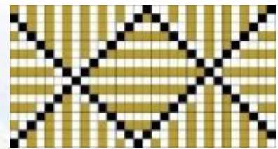
Fig 63: the new honeycomb weave structure from warp and weft on two faces with two colors for the sixth experiment
