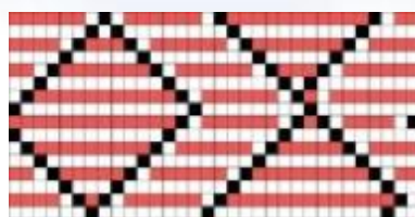
Fig 55: the new honeycomb weave structure from weft on two faces with two colors for the fifth experiment
