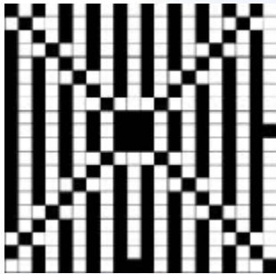
Fig 47: the new honeycomb – weave structure from warp on two faces with two colors for the fourth experiment
