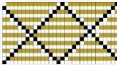
Fig 62: the new honeycomb weave structure from weft on two faces with two colors for the sixth experiment
