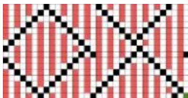
Fig 54: the new honeycomb weave structure from warp on two faces with two colors for the fifth experiment
