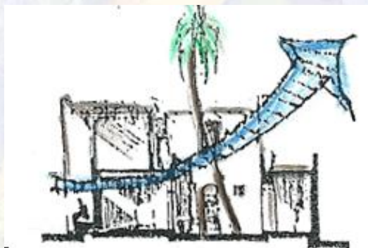
Pic.(10)shows the elevation of the proposed design with the entry and exit of mutual wind between yard and openings .
