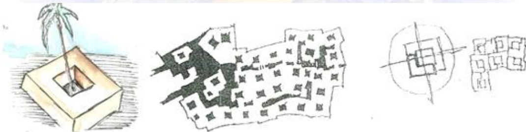
Pic.(6) shows the plan of complexes of buildings models in Bawiti city with the compact manner and the internal yard to achieve the greatest shadows.
