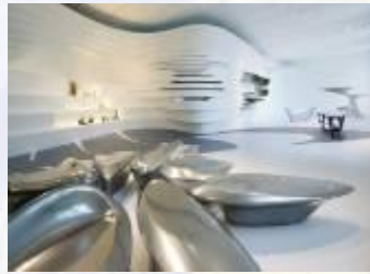
GRP in forming panels for interior and in forming furniture
