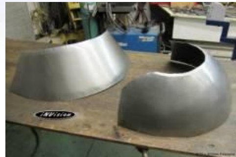
Heat and bend to form the metal
