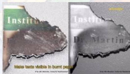
Figure 2 Using LED light produces infrared make texts visible in the right side of the photo
