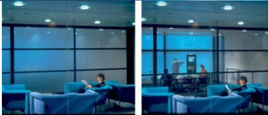
Fig (2) use of materials Alkromo electrical in the internal glass partitions to withhold the diverse activities
