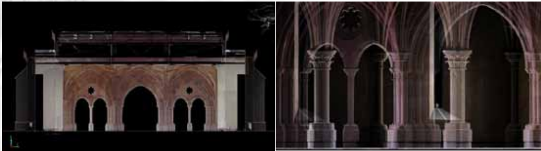
Figure 43. Sections of 3D laser scanning data.
